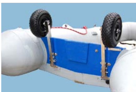
#1482 Wheel-a-Weigh Standard with 10" (26 cm) inflatable tires.
