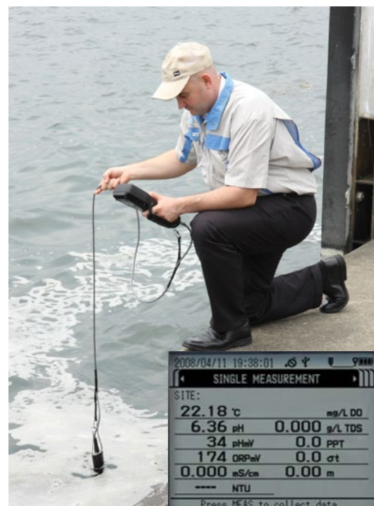
Water quality monitor displays 11 parameters simultaneously
